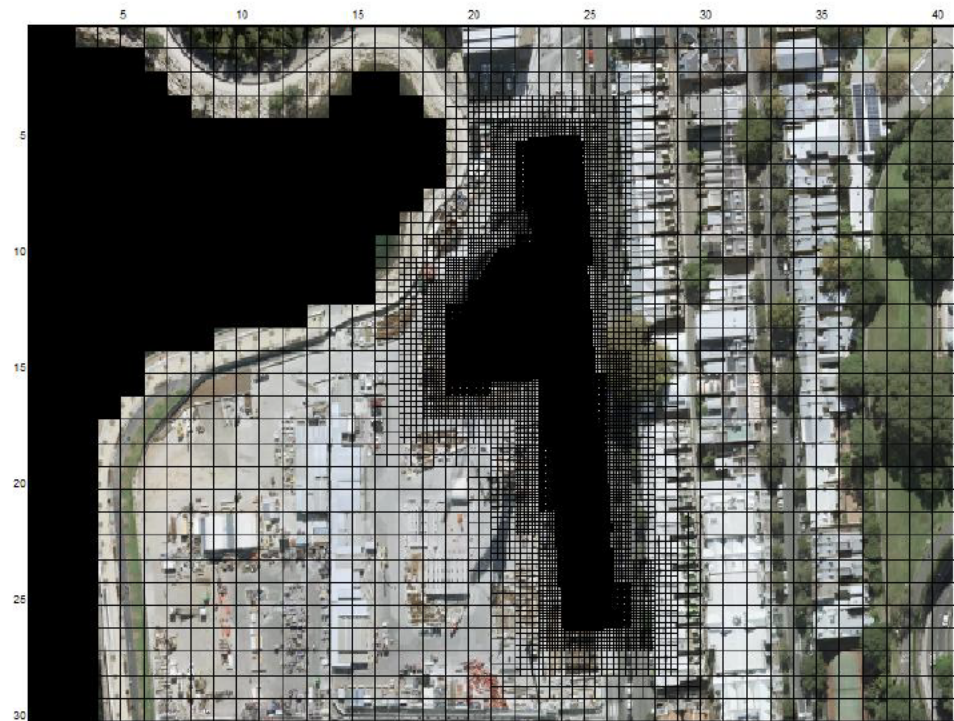
Figure 5.2 Model domain, model grid and no-flow cells (in black)
