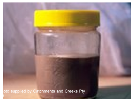
A visual example of the effect of clarifying agents in a jar test.
