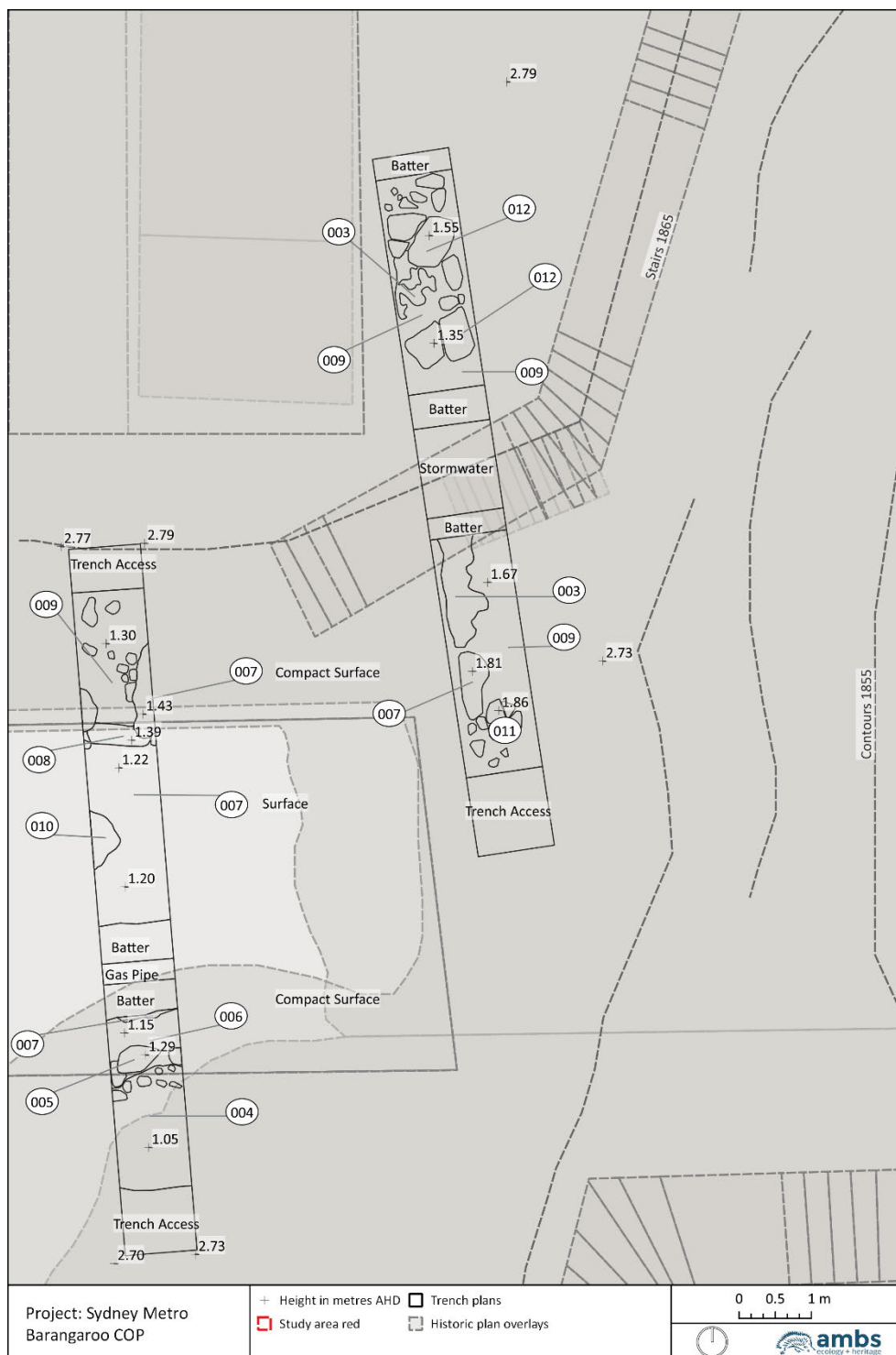
Figure 4.9: Trench 1 (left) and Trench 2.1 (right) overlain with traces of the 1834 and 1855 plans of the site showing how the features line up with the historical layout of the foreshore.
