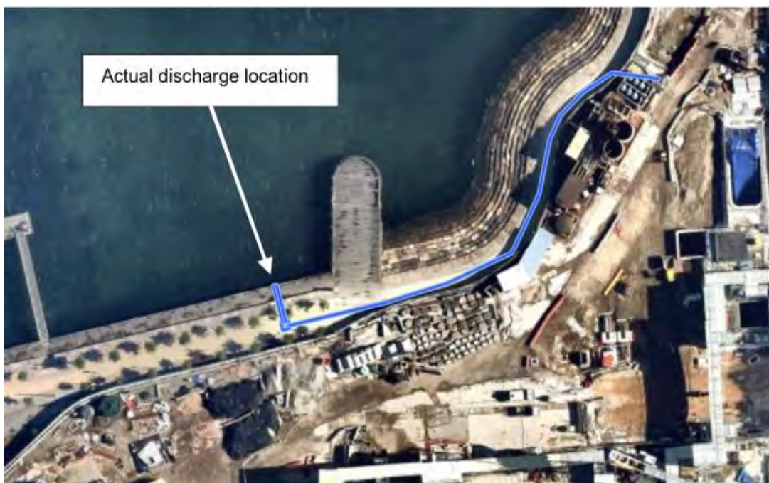
Figure 5 WTP Discharge Point through existing stormwater network
